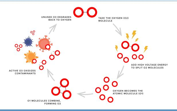
Contaminants are destroyed when **O3 oxidizes and breaks down** molecular structures. Germs and odors are eliminated and not simply covered up
